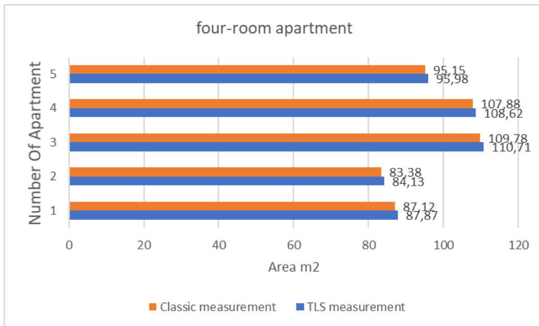
Figure 6. The resulting data of a four-room apartment according to Act - TLS measurement
